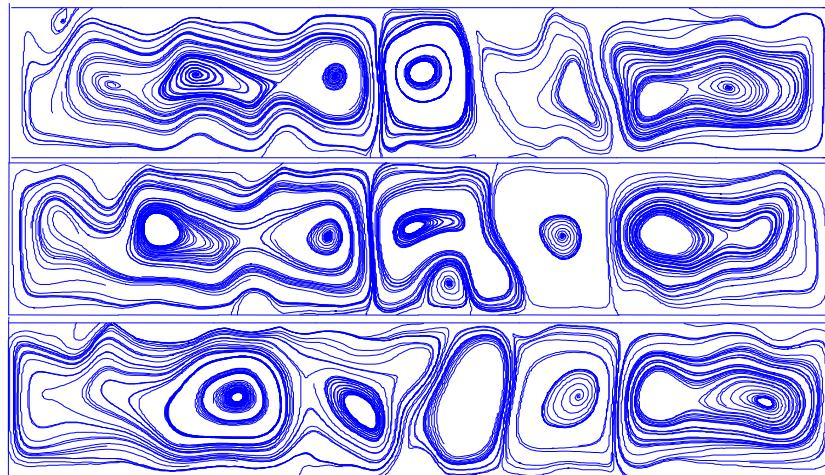
Fluid flow lines in unsteady mode of turbulent heat transfer at successive time point with 40 s intervals.
