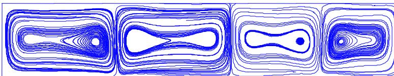
The fluid flow lines in the steady state convective heat transfer.
